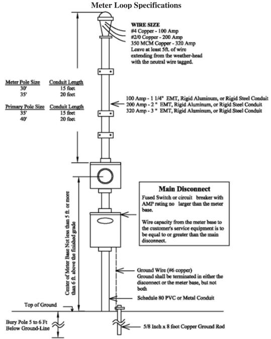
If the Member pays to have United hang the Member's meter loop, then the loop <u>MUST</u> be costructed of <u>RIGID ALUMINUM</u> (not EMT or Rigid Steel)
