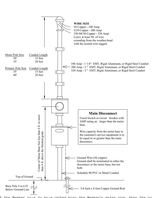
If the Member pays to have United hang the Member's meter loop, then the loop  $\underline{\text{MUST}}$  be costructed of  $\underline{\text{RIGID}}$  ALUMINUM (not EMT or Rigid Steel)
